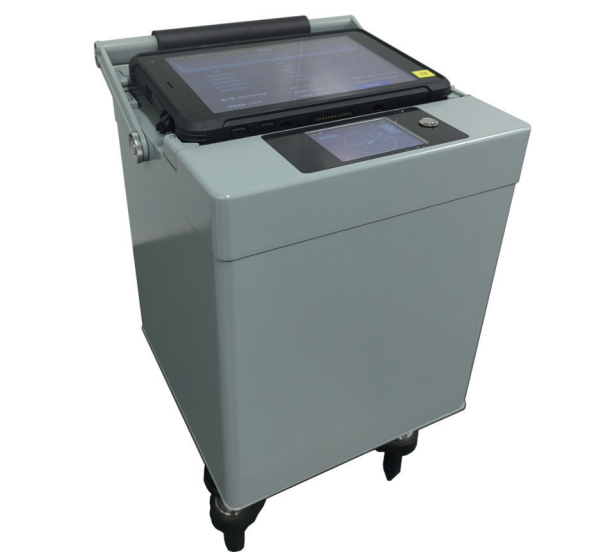
图 1 天津航海仪器研究所研制的流动式相对重力仪实物图 Fig. 1 Physical diagram of mobile relative gravimeter developed by Tianjin Navigation Instrument Research Institute
